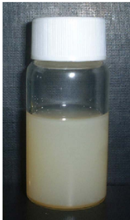
Fig. 2. Photograph of solid-in-oil (S/O) suspension prepared in this study.
